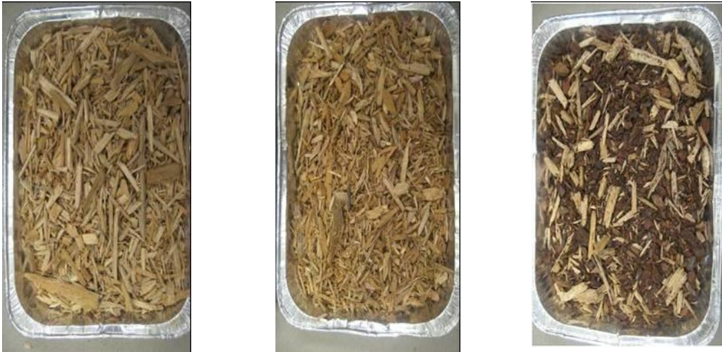
Figure 23: Samples for pelletization. From left to right: Hemlock clean white stemwood; Mix of clean white stemwood (85%)+ Rot (15%); Hemlock Bark
