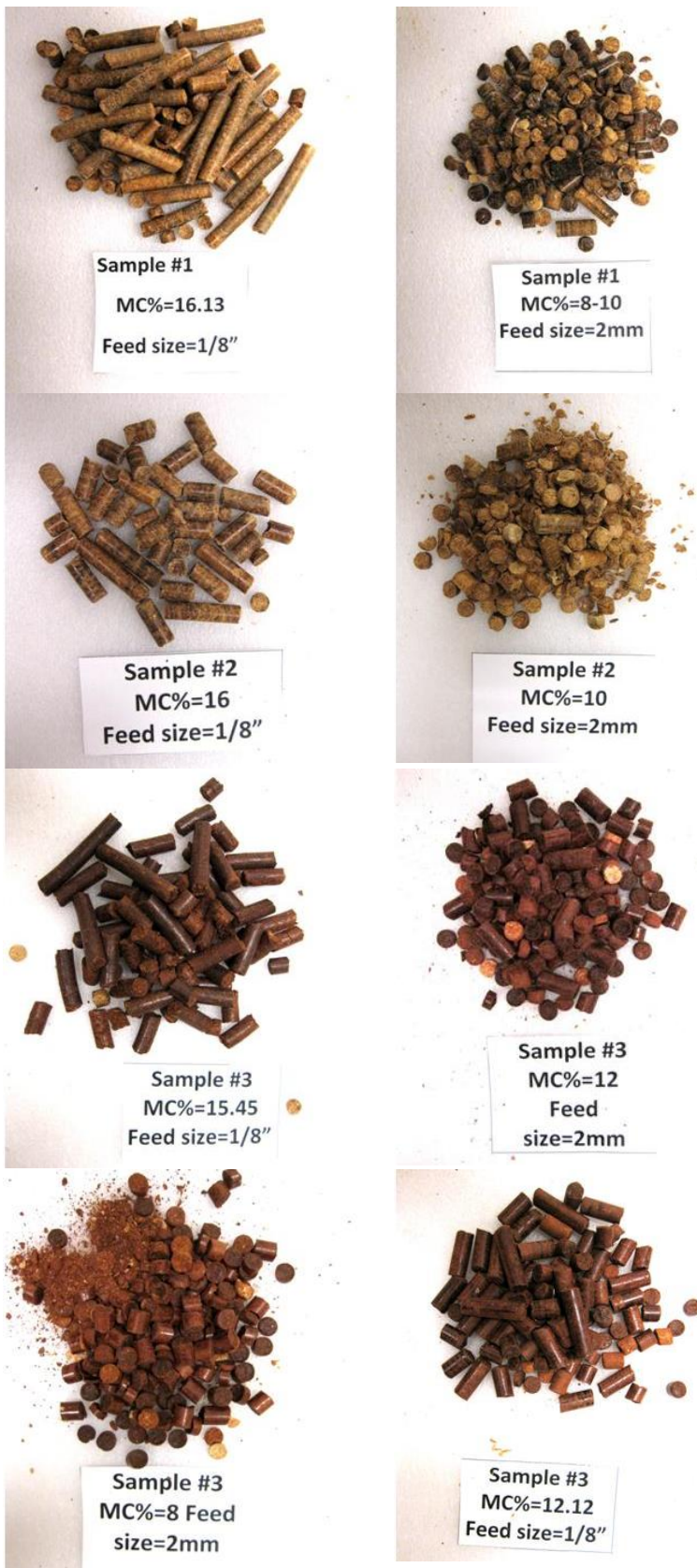
Figure 24: Pellets made from Hemloc samples: Sample 1 (Stemwood), Sample 2 (Stemwood+Rot), Sample 3 (Bark).
