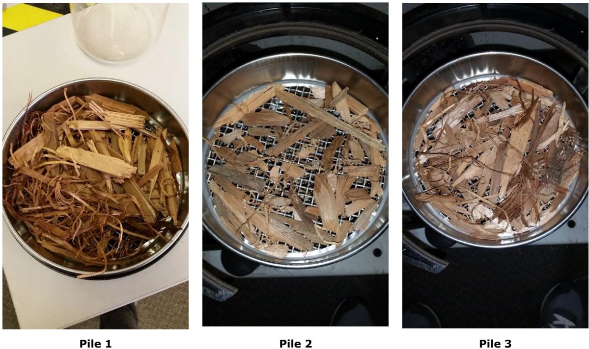
Figure 7: Size and shape of wood pieces on top sieve (6.3 mm).
